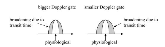
• To reduce the spectral broadening resulting from the transit time, the size of the Doppler gate (i.e., the pulse length and the beam width) may be increased to reduce the spectral width such that errors of the maximum and minimum velocity measurements can be decreased.
