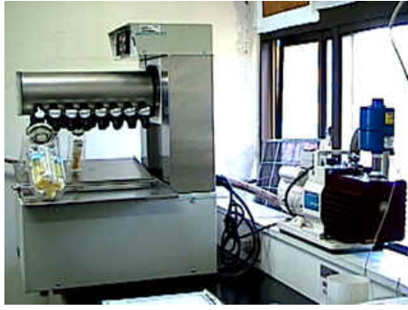
圖四：冷凍乾燥儀 (lyophilizer, Labconco, KansasCity, MO)
