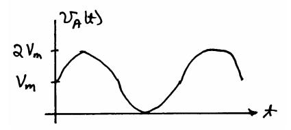
Diode  $D_2$  and capacitor  $C_2$  act as a half-wave peak rectifier. Thus, the voltage across  $R_L$  is the peak value of  $v_A(t)$ . Thus,  $v_L(t) \cong 2V_m$ . This is called a voltage-doubler circuit because the load voltage is twice the peak value of the ac input. The peak inverse voltage is  $2V_m$  for both diodes.
