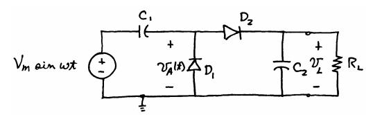
The capacitor  $C_1$  and diode  $D_1$  act as a clamp circuit that clamps the negative peak of  $v_A(t)$  to zero. Thus, the waveform at point A is:
