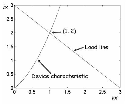
**P10.29\*** The Thévenin resistance is  $R_t = V_{oc} / I_{sc} = 10/2 = 5 \Omega$ . Also the Thévenin voltage is  $V_t = V_{oc} = 10$  V. The load line equation is  $10 = 5i_{ab} + v_{ab}$ . We plot the load line and nonlinear device characteristic and find the solution at the intersection as shown below.
