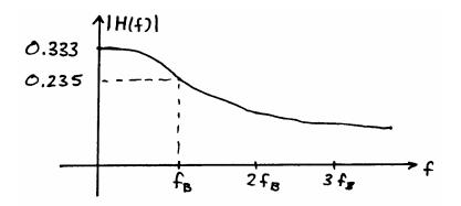
P6.39\* (a) The overall transfer function is the product of the transfer functions of the filters in cascade:
