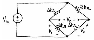
The open-circuit or Thévenin voltage is  $V_t = V_1 - V_2$ 2000 1000
