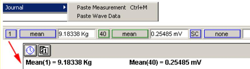
The **Paste Wave Data** function will write all the points that make up the data in the selected wave area to the Journal.
