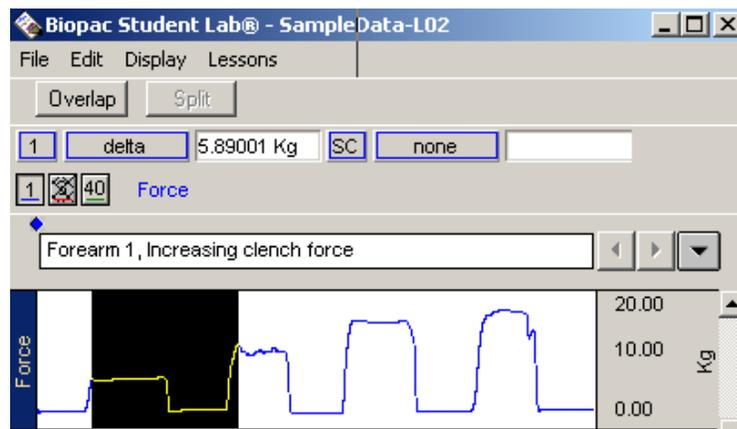
If the correct region is not established by the “**I-Beam**” cursor for the measurement type, the result will be meaningless.
