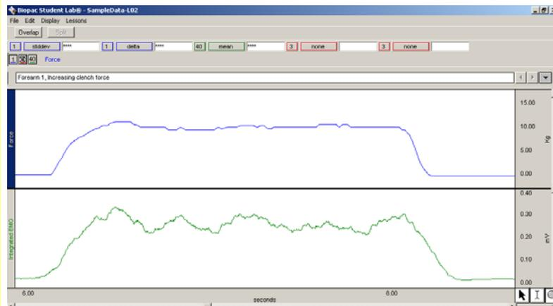
The Vertical Scale will change for the active channel only, but the Horizontal Scale will change for all channels since it (time) is the same for all channels.
