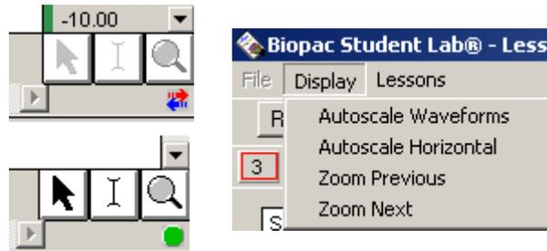
The **Arrow**, “**I-Beam**,” and **Zoom** tools are inactive (greyed) during recording but can be used between segments while in the Recording mode. The Display menu items are also available.
