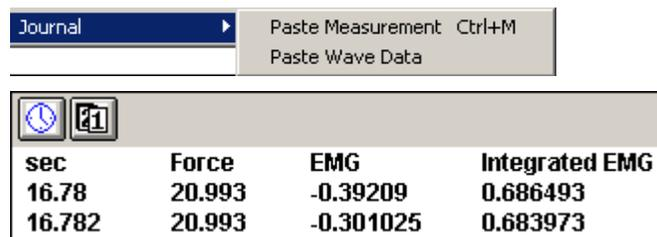
The Journal file is saved in standard text format and can be exported to word processing or spreadsheet programs—or any application that accepts Text or ASCII files.
