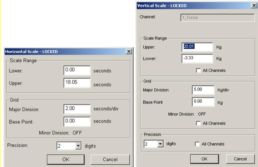
**Scale Range:** Establishes the boundary values to fit in the display window and is useful for highlighting meaningful segments in the waveform. For instance:
